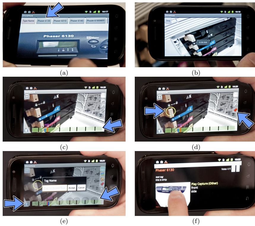
Fig. 2 Creating a tip. (a - Scan) Before shooting the video, live frames are sent to an OCR engine and then on to the server to determine the model and make of the product. The most likely model names appear as clickable icons at the top of the screen (arrow). (b - Capture & Bookmark) While recording, users can tap the screen to set a bookmark. (c - Edit & Review) While editing, the video bookmarks appear as black bars on the video timeline (arrow). Selecting a bookmark turns its bar red. (The interface for viewing a tip is similar but with editing functionality disabled.) (d) Users can add annotations to each bookmark. Here the user adds a circular region tag (left arrow). When a new annotation type is added its icon is illuminated (right arrow). (e) The user can unlock the timeline by pressing the lock icon (left arrow). The circle around each bar (right arrow) indicates its touch area. Pressing and moving a bar changes the bookmark's position in the timeline. Pressing and holding a bar lets the user set the name of its associated bookmark. On the overview screen (not shown) the user can associate tags and a more detailed text description with the entire tip and then upload all of the content to the server. (f) Immediately after uploading a video it can appear in search results.
